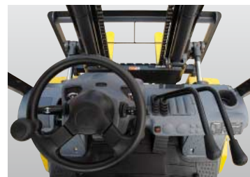
Finger-tip operation with the electric F/R lever
