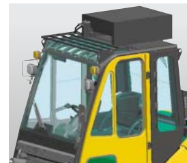
Steel cabin with cooler
