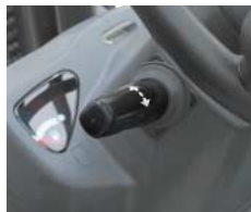
Finger-tip operation with the electric F/R lever
